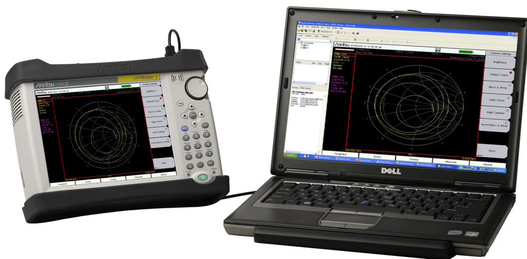
Figure 2-9. LMR Master Connected to PC via USB Mini-B
